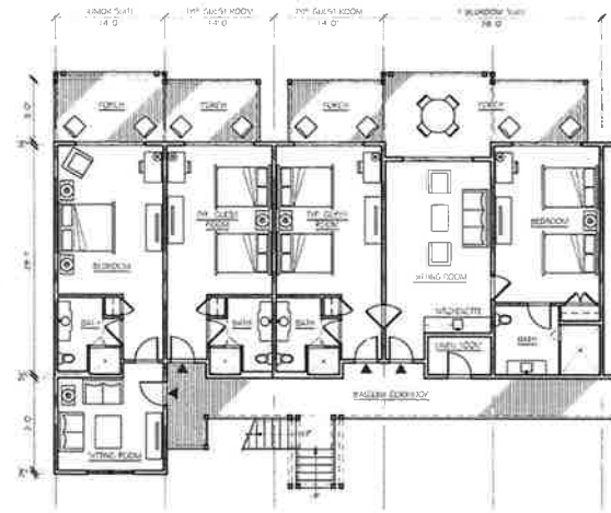
TYPICAL GUEST ROOM FLOOR PLANS SCALE: 1/8" = 1'-0"
